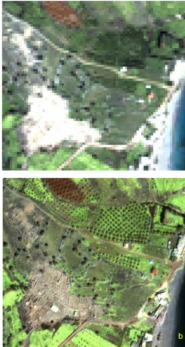
Figure 4: Comparison of enlarged 4m multispectral image (a) and 1m pan-sharpened multispectral image of the same area (b).
